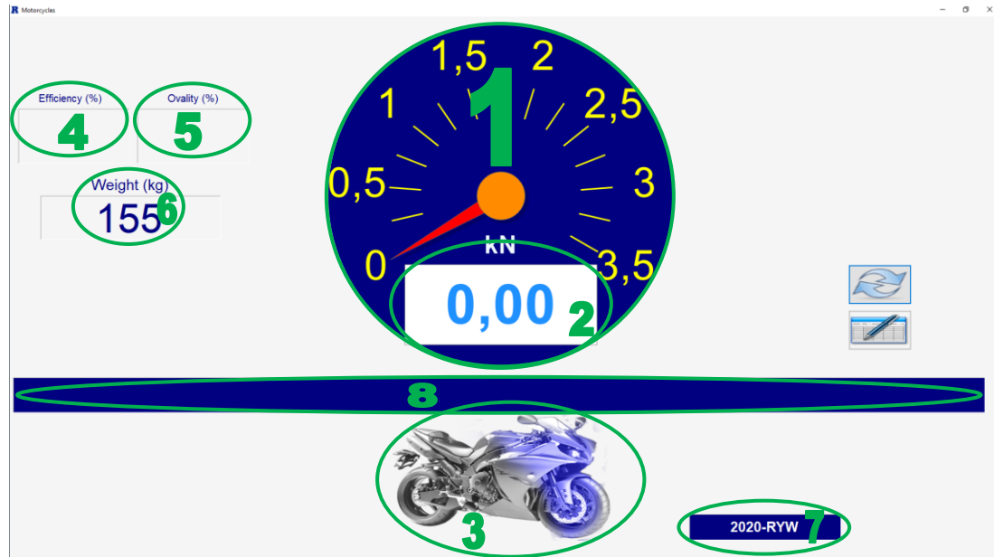
125 Motorcycles brake tester display
