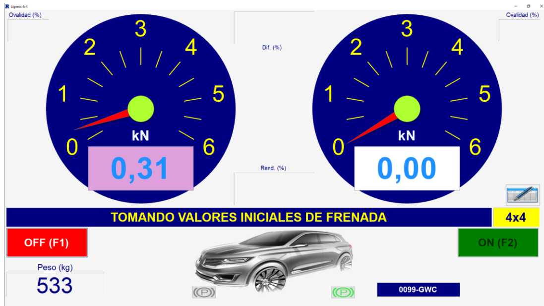
87 4x4 light vehicles brake tester: Manual mode – Residual braking measurement
