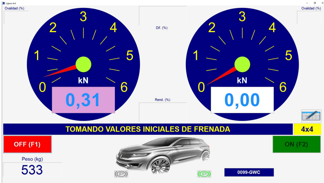
87 4x4 light vehicles brake tester: Manual mode – Residual braking measurement
